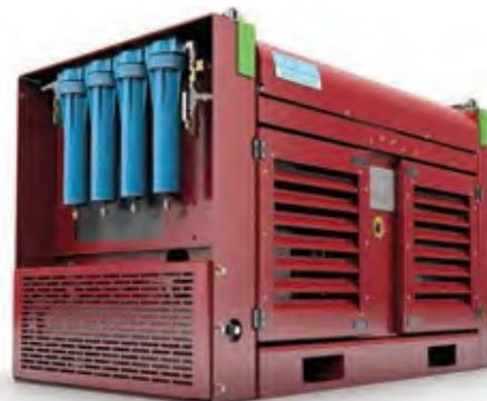
This unit takes instrument air available on the rig through air separation membranes and delivers high purity nitrogen (98 per cent) at high pressure (5000 psi).
