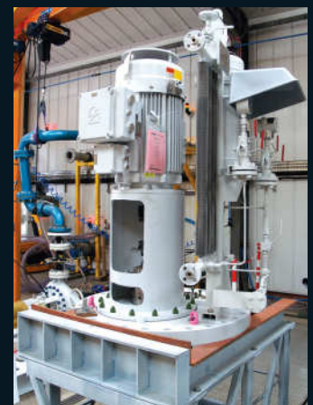
Amarinth API 610 VS4 pump with Plan 53B seal support system undergoing testing.
