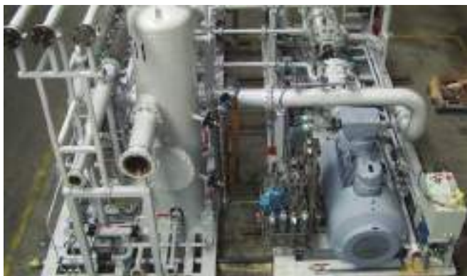
The use of a FGRS to reduce gas flaring provides environmental and social benefits
